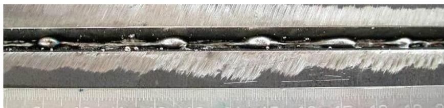
$P_L = 15 \text{ kW}$ ,  $v_s = 2.2 \text{ m/min}$ ,  $v_d = 16 \text{ m/min}$ , Böhler NiMo 1-IG
