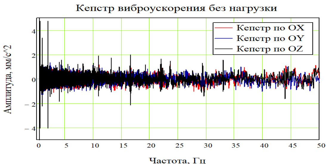
Figure 2 - Cepstre of the original signal without the introduced defect
