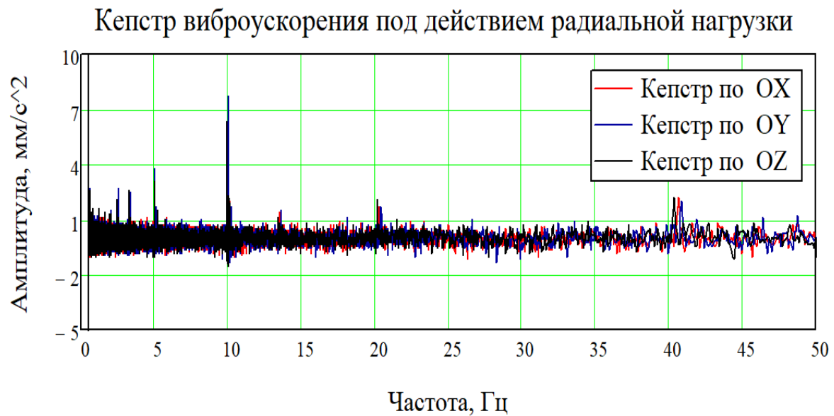
Figure 3 - Signal cepstrum with radial load imposed along the Y-axis
